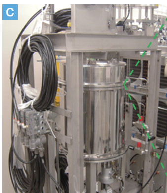
Measurement apparatus of hydrogen thermophysical properties (A) Magnetic suspension densimeter (B) Vibrating wire viscometer (C) Thermal conductivity apparatus by transient short hot-wire method
