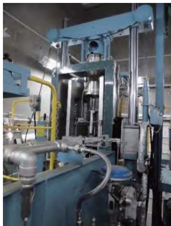
Material testing in high-pressure H_2 gas up to 140 MPa
